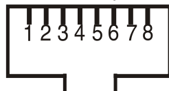
RJ-45 socket (front view):
